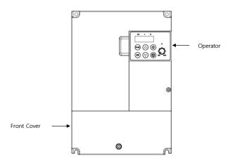
Figure 1-3 Front view with front cover
