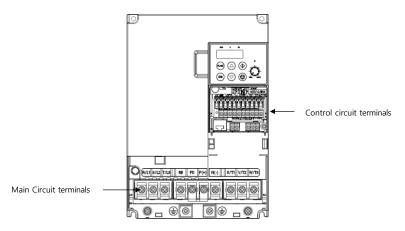
Figure 1-4 Front view without front cover
