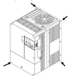
Figure 2-2 Mounting Position
