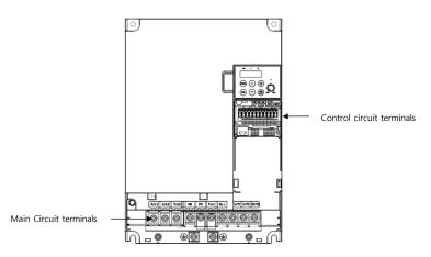
Figure 1-8 Front view without front cover
