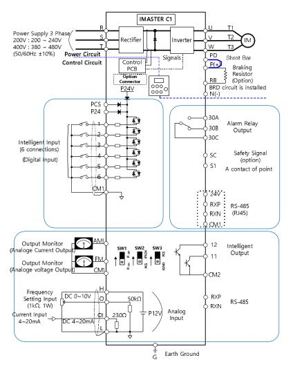
Figure 2-3 Terminal connection diagram (Sink type)
