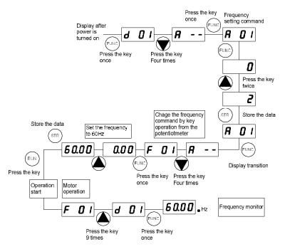
Figure 4-4 Navigation example: Mode change with arrow keypad
