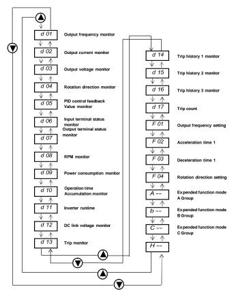
Figure 4-2 Up/Down key basic operation
