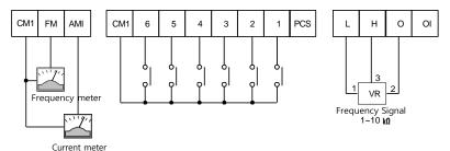
Figure 2-6 Example of control circuit wiring
