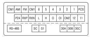
Figure 2-5 Control circuit terminal
