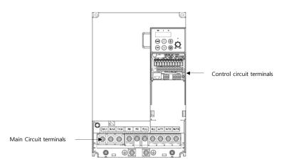
Figure 1-6 Front view without front cover
