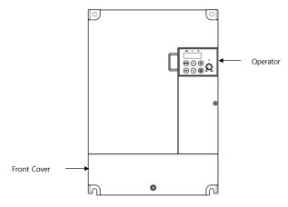
Figure 1-7 Front view with front cover
