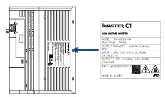
Figure 1-2 iMaster C1 Specification on label
