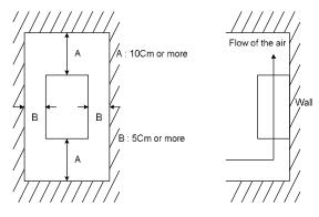
Figure 2-1 Air gap (Installation)
