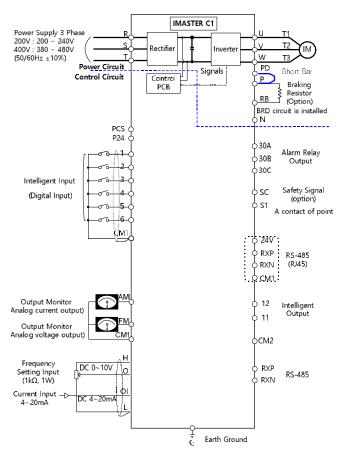
Figure 4-6 Setting diagram from the terminal
