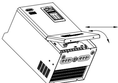
**Fig.3-5 Metal cover disassembly and assembly**
