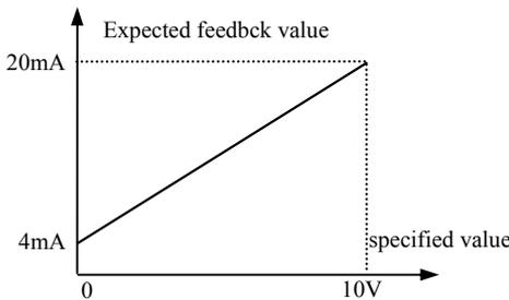
**Fig.6-15 specified value and expected feedback value**
