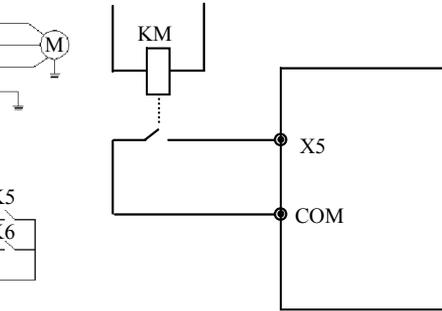
**Fig.6-26** exterior device failure always-open input
