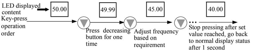
**Fig. 4-8 set frequency adjustment operation example**
