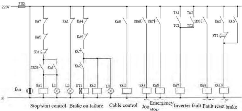
Note: Ansprechstrom current of intermediate relay KA6、KA8 should not more than 30mA, otherwise, please use external power.
