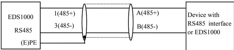
**Fig.3-15 Communication terminal wiring**
