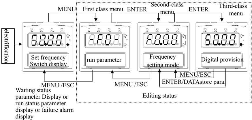
**Fig.4-5 keypad display status switching**
