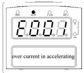
**Fig.4-4 failure alarm**
