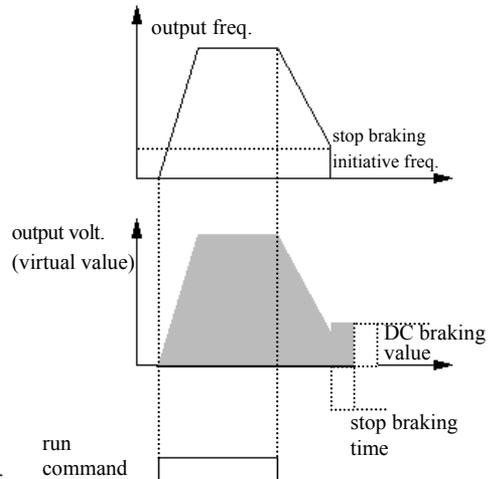
**Fig.6-8 Dece stop+DC braking**
