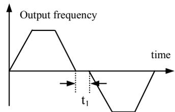
Fig.6-9 FWD REV run dead-section time
