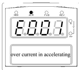
Fig.4-4 failure alarm
