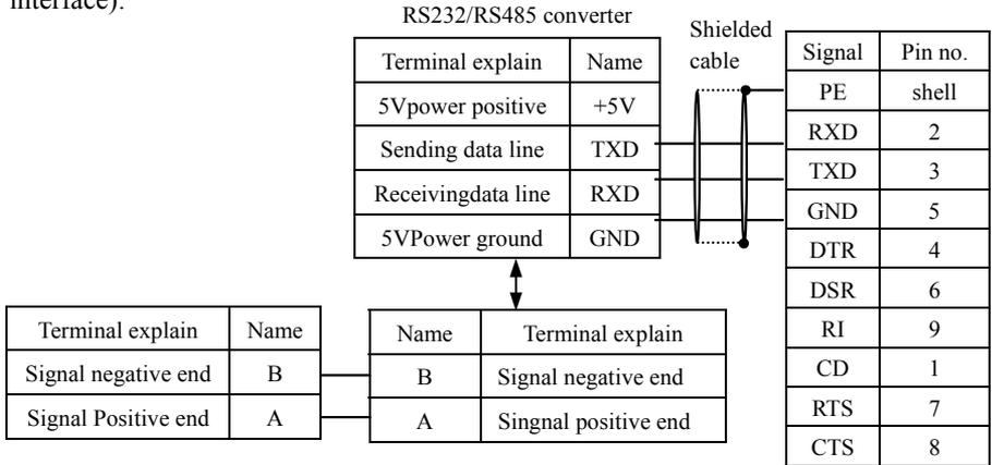
**Fig. 3-16 RS485 communication wiring**
