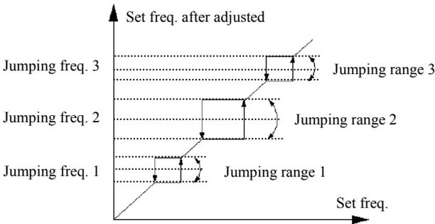
**Fig.6-12 jumping frequency and range graph**
