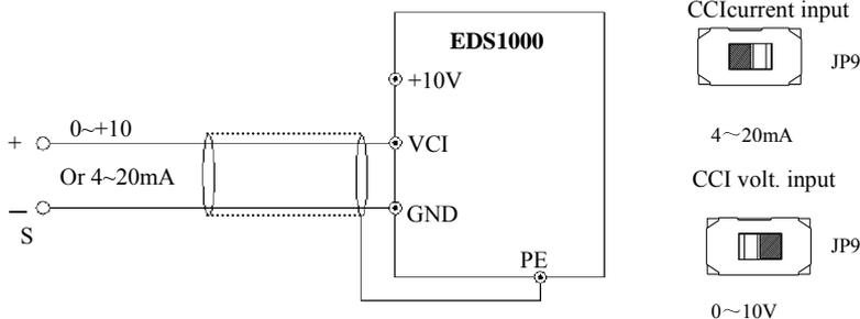
**Fig.3-12 CCI terminal wiring diagram**
