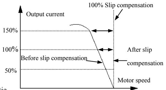
**Fig.6-10 slip freq. compensation graph**
