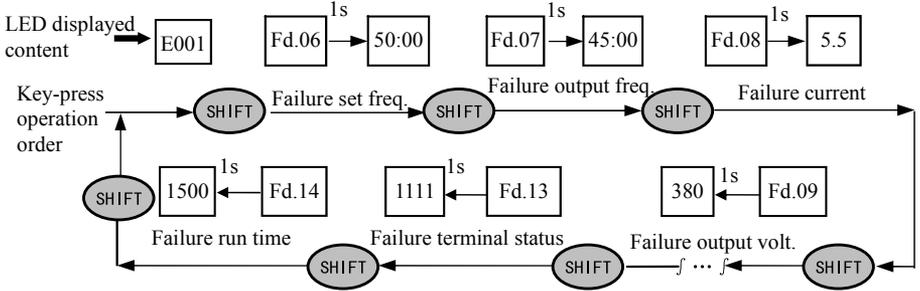
**Fig.4-11 failure status searching operation example**
