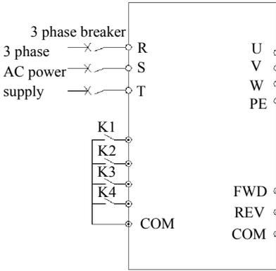
**Fig.6-25** multi-step speed run
