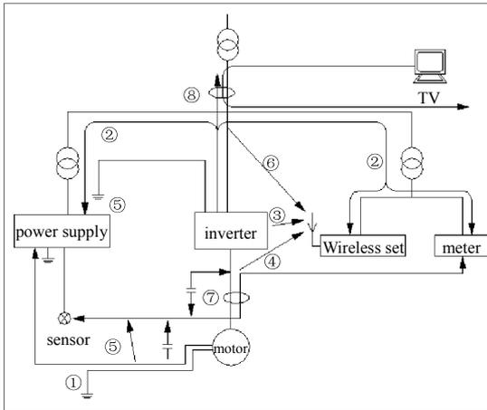
**Fig.3-19 noise disturbance spread road sketch**
