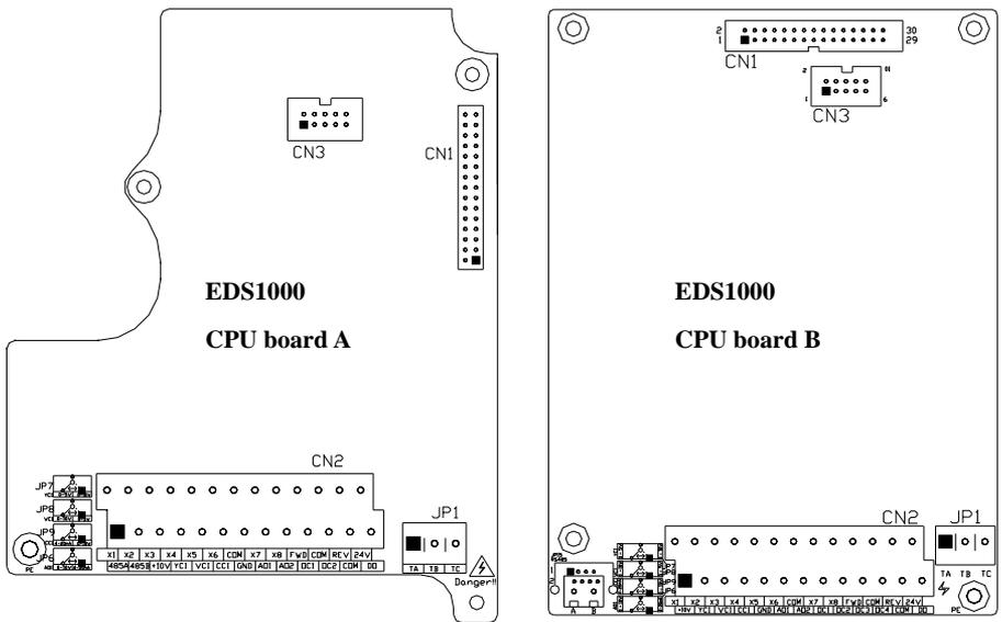
Fig. 3-10 slide switch on CPU board
