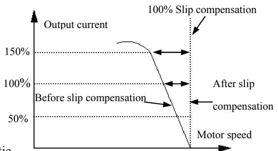
**Fig.6-10 slip freq. compensation graph**
