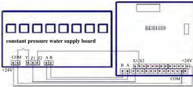
**Fig.10-7 connection between water supply controller and inverter**
