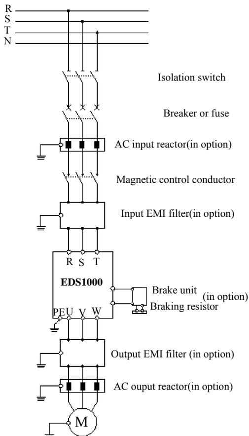
Fig.3-8 connection of inverter and fitting parts
