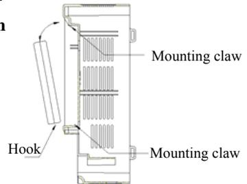
**Fig.3-3 mounting sketch of keypad**
