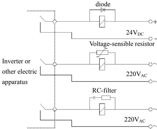
**Fig.3-21 installation demand for electromagnetic on-off device**
