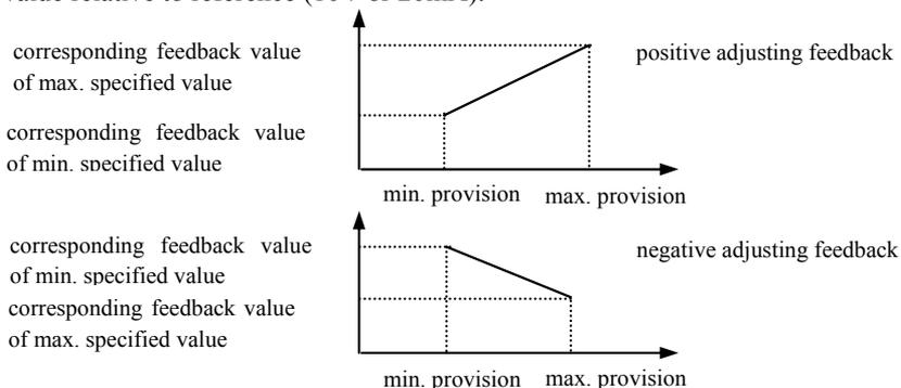
**Fig.6-16 provision, feedback curve**
