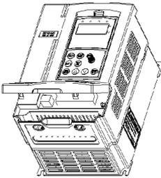
**Fig. 3-4 disassembly and mounting sketch of plastic cover**
