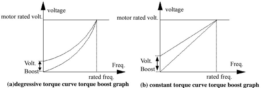
**Fig.6-4 torque boost graph**
