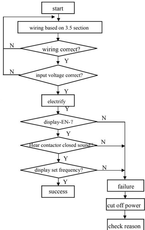
Fig. 4-12 first electrification operation flow
