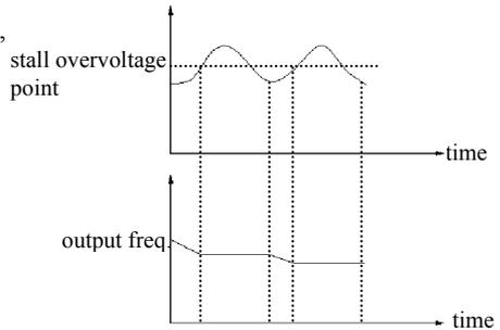
**Fig.6-38 overvoltage stall function**
