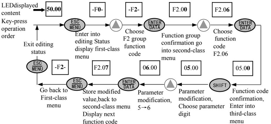
**Fig.4-7 example for parameter setting and modification**
