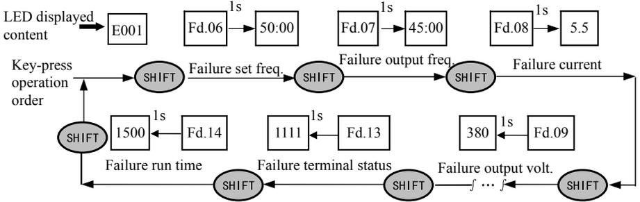
**Fig.4-11 failure status searching operation example**
