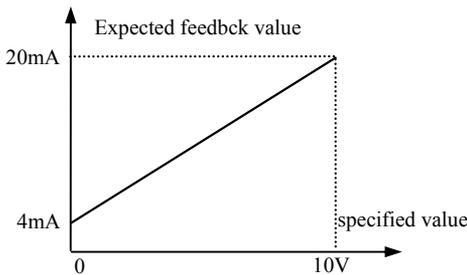
**Fig.6-15 specified value and expected feedback value**
