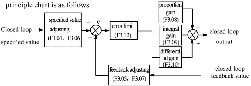
**Fig.6-14 PID control principle diagram**
