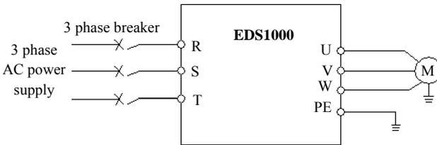
**Fig.3-7 main loop simple wiring**
