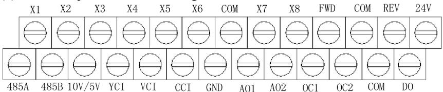
(2) control loop terminal CN2 arranged as follows for inverter above 2.2kw:
