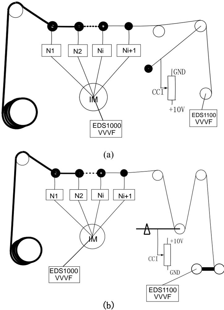
Diagram 1-1 Drawing machine with retracting and releasing volume diagram
