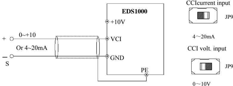
**Fig.3-12 CCI terminal wiring diagram**
