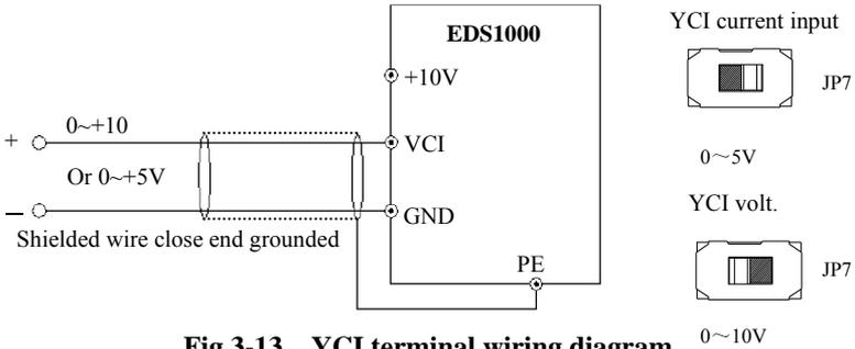
**Fig.3-13 YCI terminal wiring diagram**
