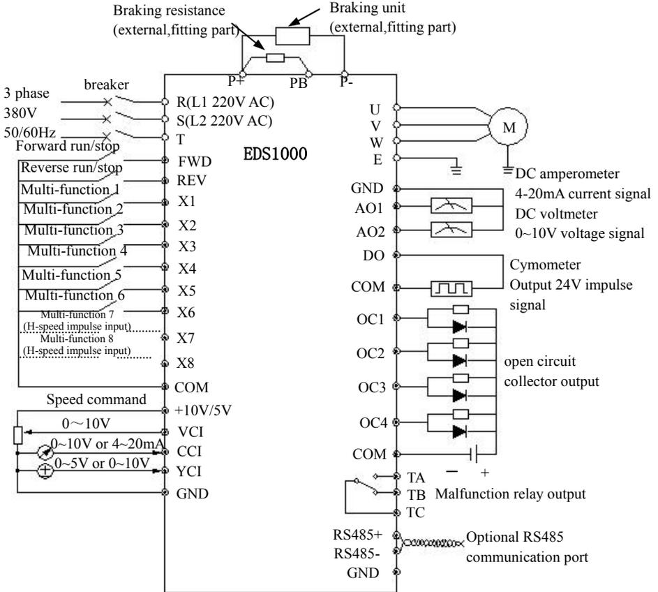
Fig. 3-9 basic wiring diagram
