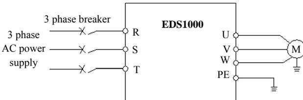
**Fig.3-7 main loop simple wiring**
