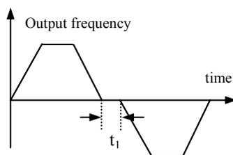
Fig.6-9 FWD REV run dead-section time
