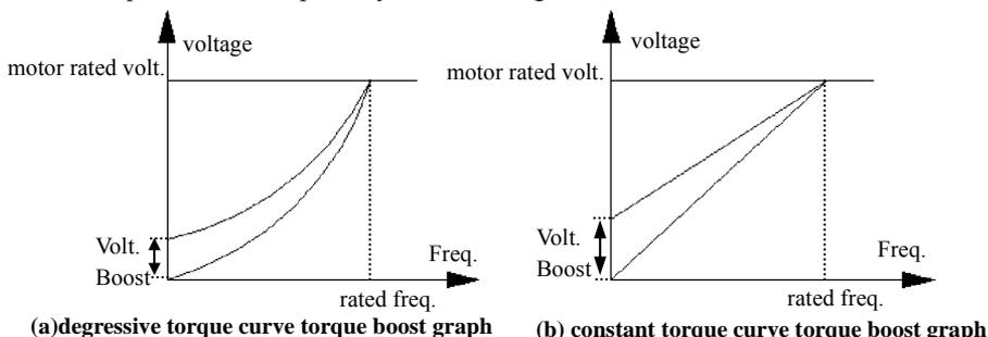
**Fig.6-4 torque boost graph**
