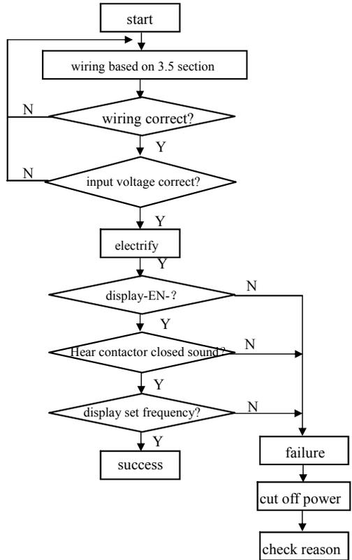
Fig. 4-12 first electrification operation flow
