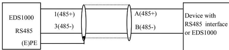
**Fig.3-15 Communication terminal wiring**
