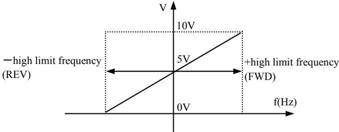
2> when YCI input voltage is 0~5V:
