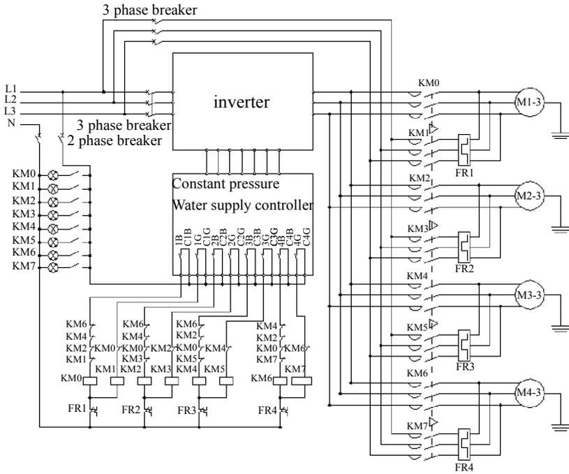
**Fig.10-10 basic wiring diagram for constant pressure water supply controller**
