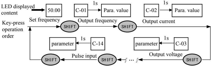
**Fig. 4-6 waiting status parameter display operating example**
