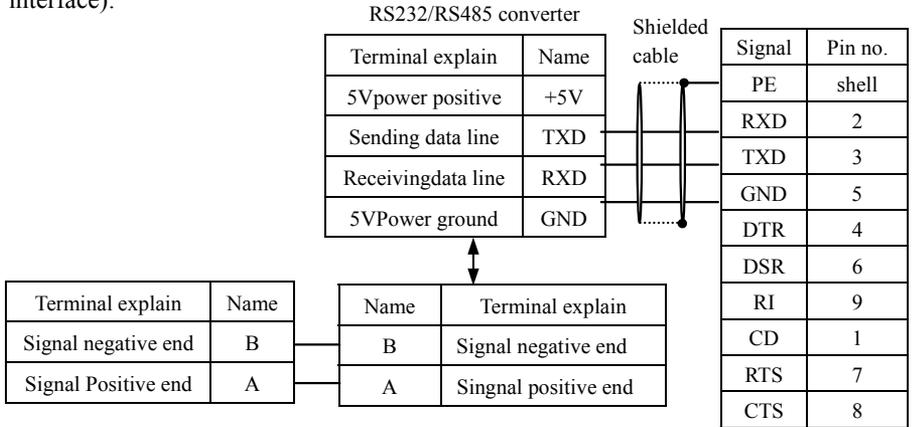
**Fig. 3-16 RS485 communication wiring**
