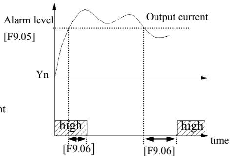
**Fig.6-36 electronic thermal relay protection Fig.6-37 overload alarm**
