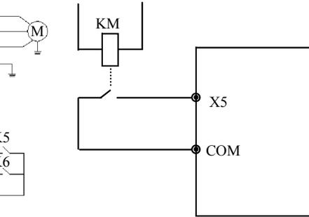
**Fig.6-26** exterior device failure always-open input
