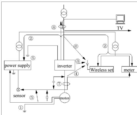
**Fig.3-19 noise disturbance spread road sketch**
