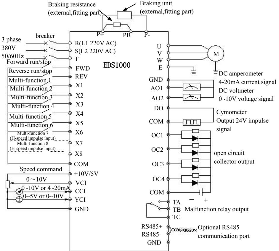
Fig. 3-9 basic wiring diagram
