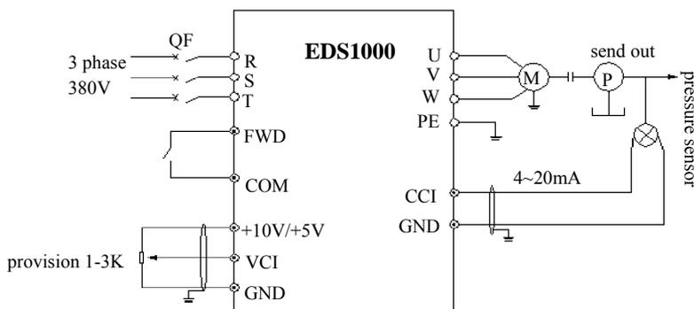
**Fig.6-13 built-in PID analog feedback control system graph**
