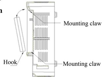
**Fig.3-3 mounting sketch of keypad**
